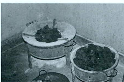
Charcoal-saving stove (insulated bricks)
