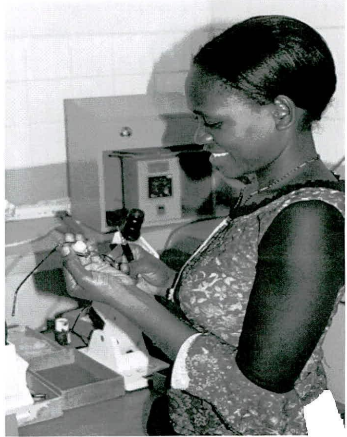
Making spectacles in Lira – putting lenses in the frames
